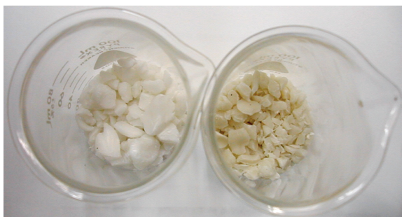
Figure 9. Photography of PP/PS (85:15) blends processed without compatibilizer, right side, and processed with 0.03 phr of the SBS compatibilizer, left side.
