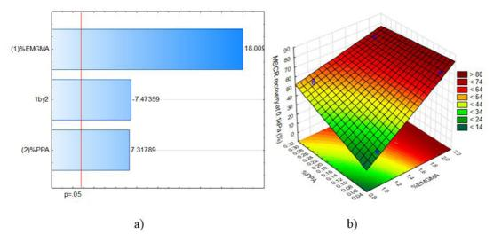
Figure 9. MSCR recovery at the stress of 0.1 kPa (a) Pareto chart and (b) response surface.
