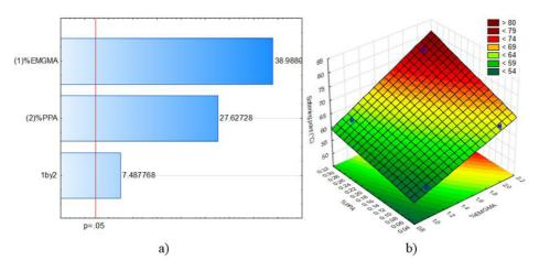
Figure 5. Softening point (a) Pareto chart and (b) response surface.
