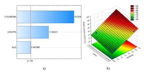
Figure 6. Elastic recovery at 25°C (a) Pareto chart and (b) response surface.
