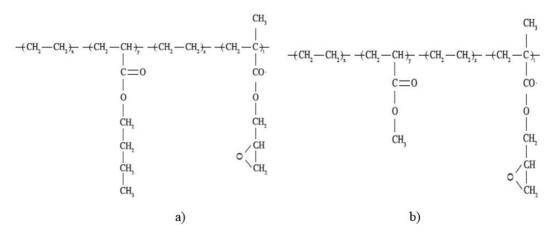
**Figure 2.** Molecular structure of (a) ethylene-butyl acrylate-glycidyl methacrylate terpolymer and (b) ethylene-methyl acrylate-glycidyl methacrylate terpolymer (adapted from Brito et al.<sup>[11]</sup>).
