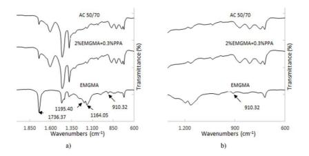
Figure 15. (a) FTIR spectrum of unmodified asphalt binder, pure EMGMA and the sample 2%EMGMA+0.3%PPA; (b) zoom for the epoxy groups.
