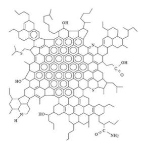
Figure 1. 2-Dimensional model of an asphaltene molecule<sup>[10]</sup>.
