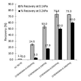
Figure 8. MSCR recovery percentage at stresses of 0.1 kPa and 3.2 kPa.
