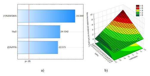
Figure 11. Non-recoverable compliance  $(J_{uv})$  at the stress of 0.1 kPa (a) Pareto chart and (b) response surface.
