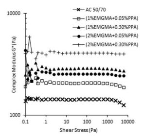
Figure 12. Modulus complex G\* as function of the shear stress for the samples tested at 64°C.
