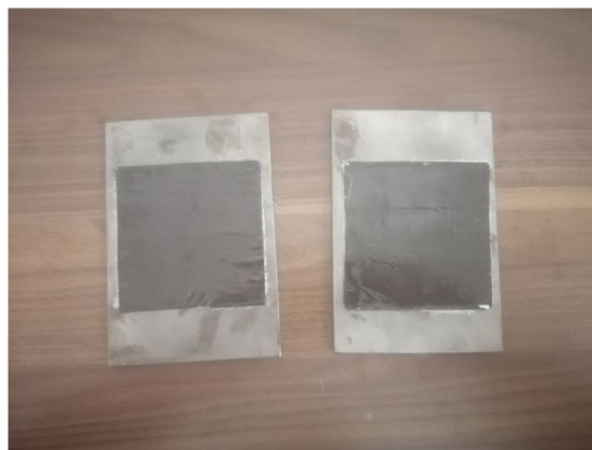
Figure 4. Hybrid woven glass and carbon reinforced epoxy blister test samples with and without nano reinforced adhesives.
