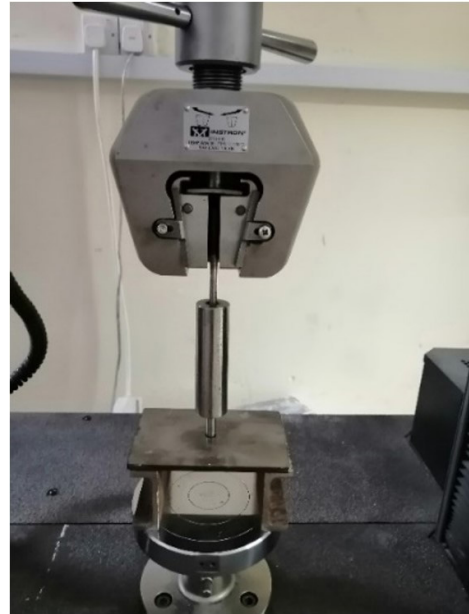
Figure 5. Sample of blister test in Instron machine.
