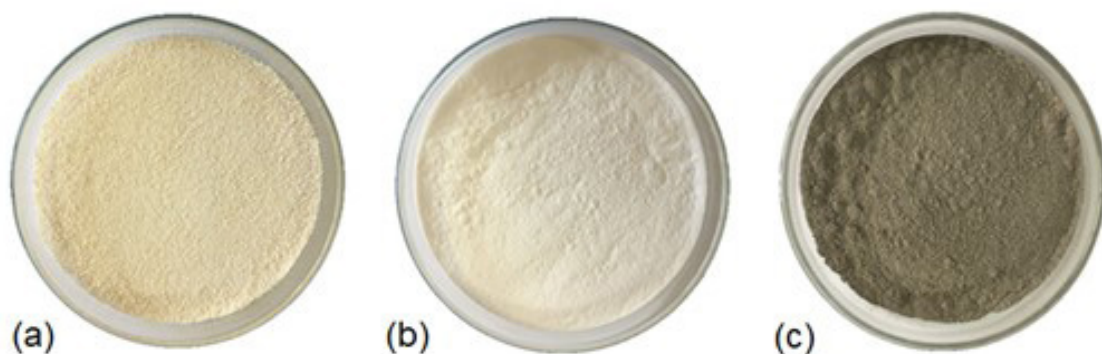
Figure 1. (a) ground eggshell; (b) in natura powder; and (c) the bio- \text{CaCO}_3 .
