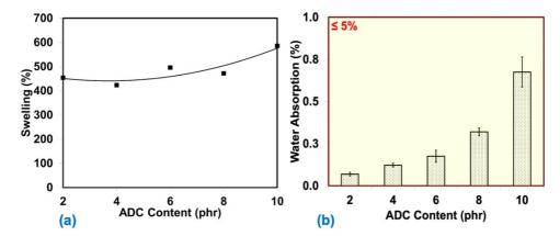
Figure 4. Swelling uptake (a) and water absorption (b) of NRF prepared by various ADC content.
