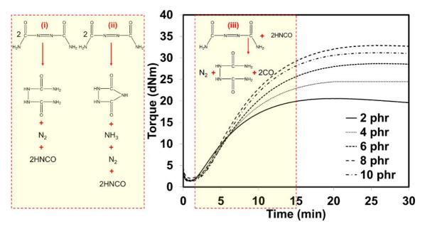
Figure 2. Chemical decomposition of ADC and rheometric curves of NRF prepared by various ADC content (The reaction schemes were adapted from Reyes-Labarta and Marcilla<sup>[15]</sup>.
