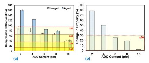
Figure 5. Compression-deflection before and after thermal aging (a) and their corresponding change in property (b) of NRF prepared by various ADC content.
