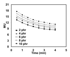
Figure 1. Mooney viscosity of NRF prepared by various ADC content.
