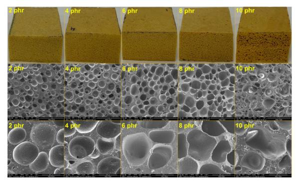
Figure 3. Optical image (top) and SEM images at 50× (middle) and 300× (bottom) magnifications of NRF prepared by various ADC content.
