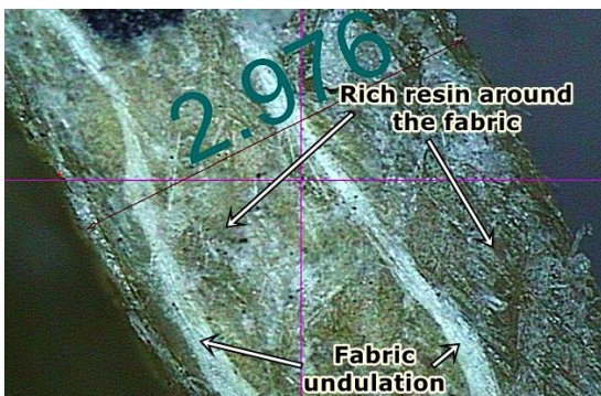
Figure 12. Microscopic image of the specimen at the flange.
