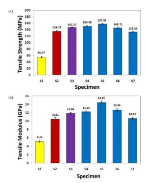
**Figure 2.** (a) Variation of Tensile Strength with the different Compositions; (b) Variation of Tensile Modulus with the different Compositions.
