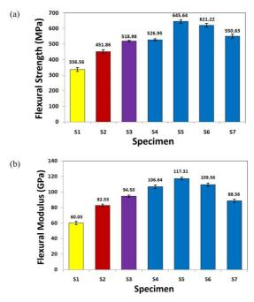
**Figure 3.** (a) Variation of Flexural Strength with the different Compositions; (b) Variation of Flexural Modulus with the different Compositions.
