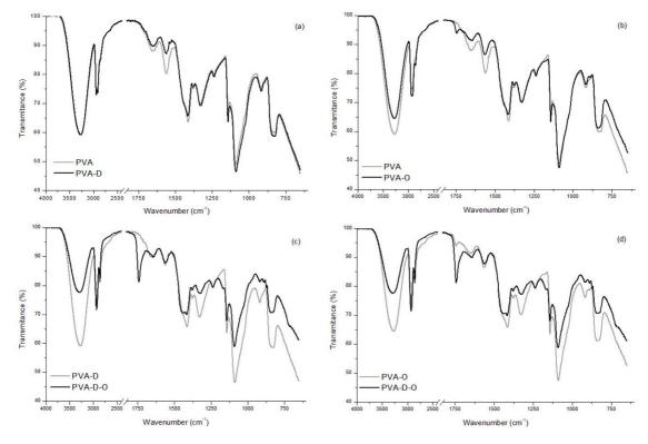
Figure 1. FTIR spectra of the samples: (a) PVA and PVA-D; (b) PVA and PVA-D; (c) PVA-D and PVA-D-O; (d) PVA-O and PVA-D-O.
