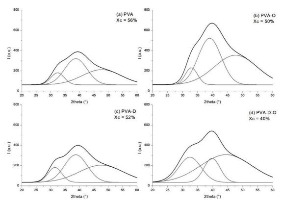
Figure 2. XRD deconvoluted curves of the samples: (a) PVA; (b) PVA-O; (c) PVA-D and (d) PVA-D-O.
