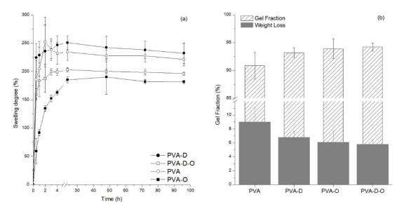
Figure 3. (a) Samples swelling degree and (b) Gel fraction and Weight loss.
