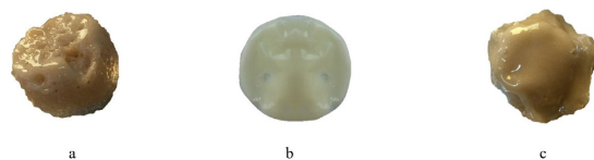
Figure 6. Polyurethane obtained from OOHT (a), from CBHT (b) and from ALHT (c).
