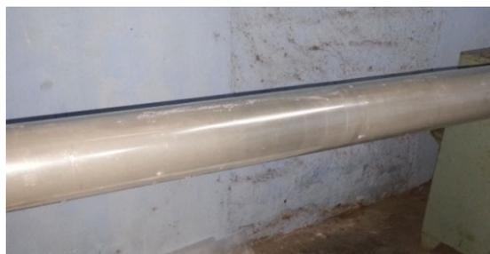
Figure 1. Terphane releasing film wounded mandrel.
