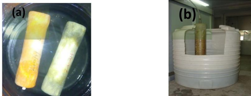
Figure 3. (a) Burst pressure test specimens (b) Specimen in connector & placed in closed location.
