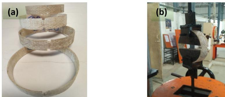
Figure 4. (a) shaped specimens (before test) (b) specimen in ring test kit.
