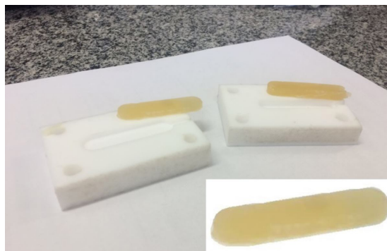
Figure 4. Photography of polyurethane castor oil (COP) resorbable plates, with dimensions of 40\text{ mm} \times 10\text{ mm} \times 2\text{ mm} .
