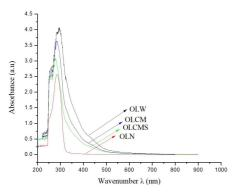
Figure 8. Visible spectrum absorbance of new lubricating oil (OLN), clarified lubricating oil with melamine silica (OLCMS), clarified lubricating oil with melamine (OLCM) and waste lubricating oil (OLW).
