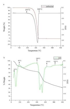
**Figure 7.** TG/DTG thermal analysis curves of the materials. Melamine in 7.a and MS in 7.b.
